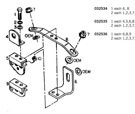
**NOTE:** Any space between upper mount (6) and frame mount plate should be closed up by using washers as per factory manual
