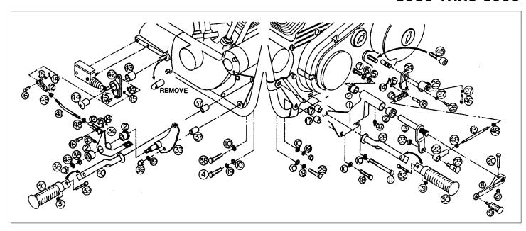
NOTE: Use blue Loctite on first three threads of all hardware!
