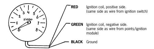
Connect tacho light wire with speedo or taillight wire.
