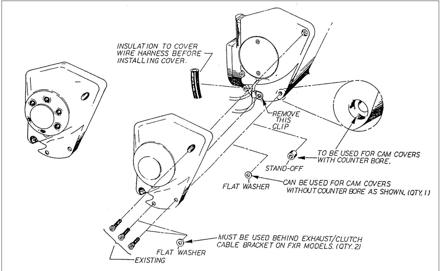
These covers are designed to fit over the existing cam covers on 1970 thru 1999 Single Cam Big Twin models. Due to variances in OEM cam cover castings from year to year, the supplied spacer and washers will be needed to ensure the best possible fit and spacing.
