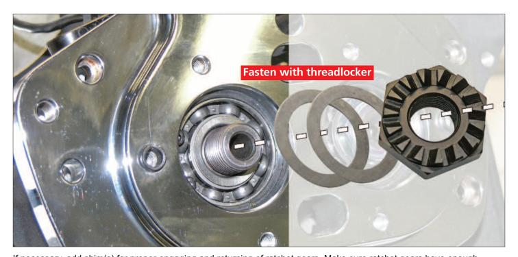
If necessary, add shim(s) for proper engaging and returning of ratchet gears. Make sure ratchet gears have enough clearance so they do not touch when not engaged.
