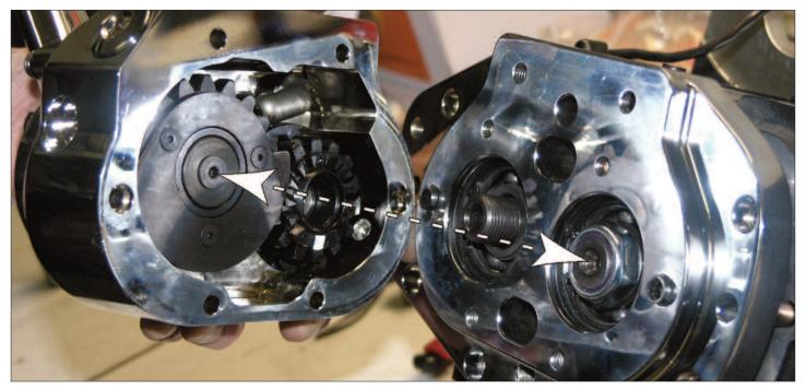
Check for proper clearance between counter shaft and counter sunk allen bolt.
