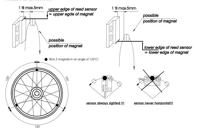
Install the sensor and the magnets according to the sketch. The mentioned dimensions refer to the reed sensor of NOVA-MMB.
