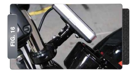
Figure 15 and Figure 16 are examples of the Power Vision module mounted to a 2009 Night Rod using the Techmount bracket.
