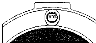
FRONT CYLINDER 20° MARK DO NOT USE
