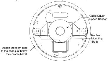
Mounting hardware for the clip-in system with an electric, transmission speed sensor.
