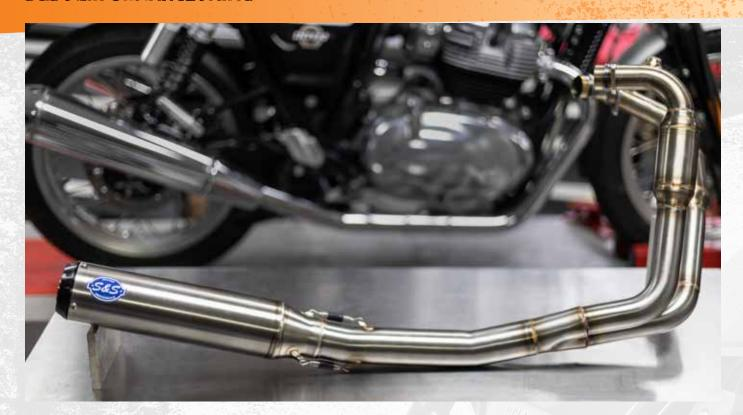
The Qualifier is an aggressively styled 2-1 race replica exhaust system built for 2019-2020 RE 650 models. Crafted from TIG welded brushed stainless steel, it's as durable as it is good looking and sheds a full 28 lbs over the stock system. More importantly it bumps horsepower 12% and torque 7% while emitting a deep race note that's just as happy on the track as it is on the street.
